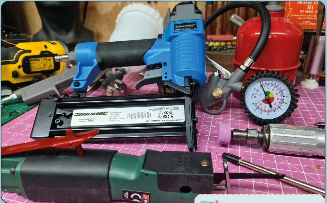
Above ♦ Not every power tool is a battery tool. Don't discount the idea of air tools – they can be cheaper, faster, more powerful, and quieter than their electric equivalents if you already have a compressor
