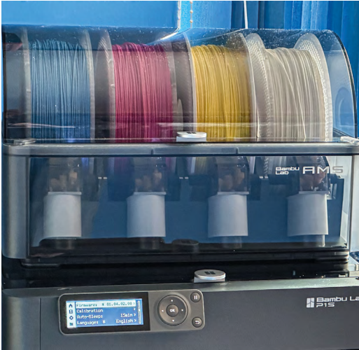
Figure 2 ♦ The selector has been loaded with cyan, magenta, yellow, and white filaments to make a colour lithophane
