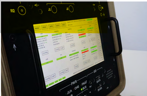
Below ↓ Main panel showing all subsystem data and status
