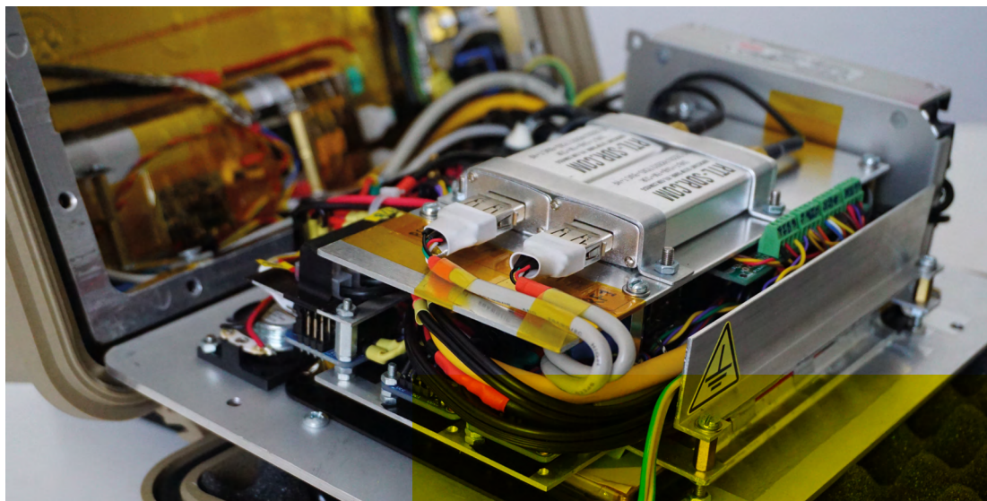
Left ← Side view of the finished stack showing the two RTL-SDR receivers on the top
