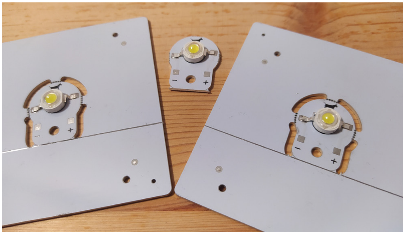
Figure 6 ♦ Our small aluminium LED module
