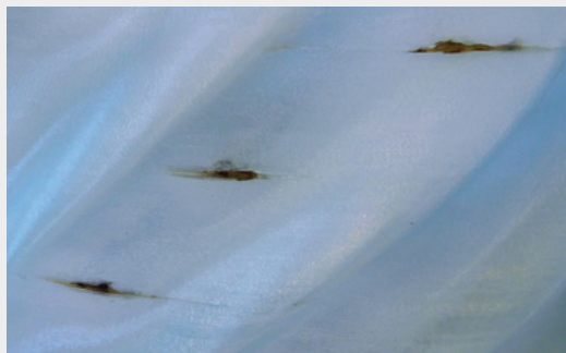
Above ◆ Blobs of nylon can stick to the nozzle, burn, and then detach onto the print leaving scorch marks
