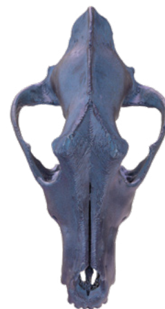
Above We printed this wolf skull upside down so that the teeth would print without supports. Unfortunately, this has left it with a messy area on the top of the skull
