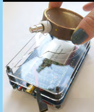
Above ◆ Installing the pancake Geiger-Müller sensor into the bGeigie Nano
