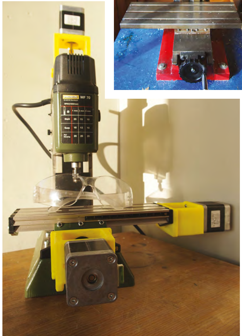
Figure 2 ♦ Perhaps the smallest milling machine is the tiny Proxxon MF 70. This one is currently being modified into a CNC milling machine
