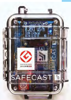
Below ♦ A fully assembled bGeigie Nano kit, housed inside a Pelican hardshell
