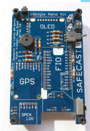
Above ♦ The main board of the bGeigie Nano
