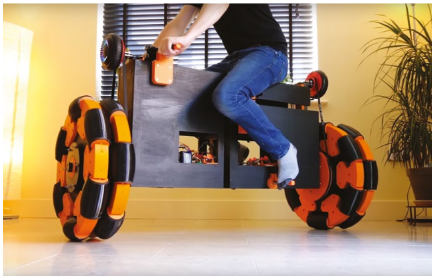
Right ▣ The bike uses ommissions wheels; next time James is going to try mecanum wheels, last seen in HackSpace issue 71
