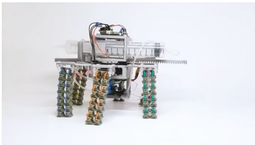
Right □ This soft robot can walk at a speed of 0.05 body lengths per second, and can also crouch
