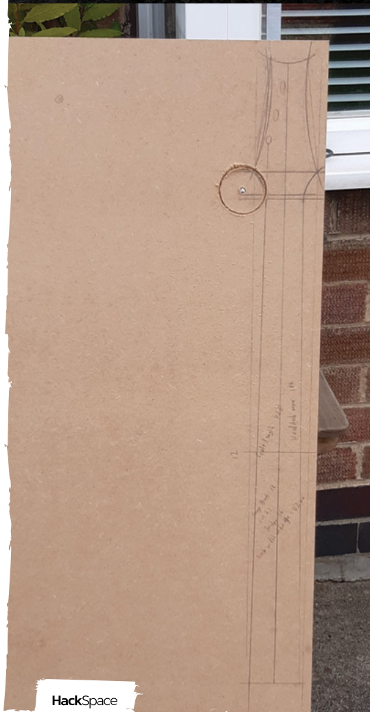
Above ◀ By trial and error, I've managed to get the cutting slot exactly the right length for my truss-rod, which should mean fewer trials and less error in future
