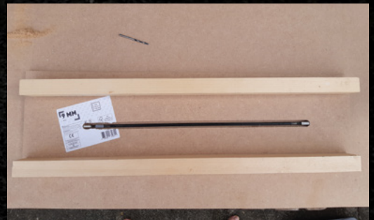
Left ◀ MDF isn't the most pleasant material to work with; it blunts tools, it looks dull, and it kicks up a load of toxic dust when you cut it with power tools. The advantage it has is that it doesn't warp, and it's relatively cheap
