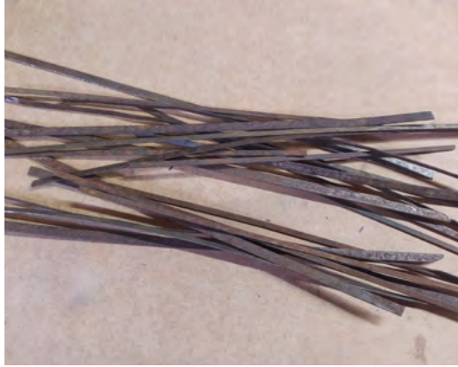
Figure 3 ♦ Although it may seem a strange hobby, collecting broken street-sweeper bristles provides an excellent stock of materials for making a variety of locksport tools
