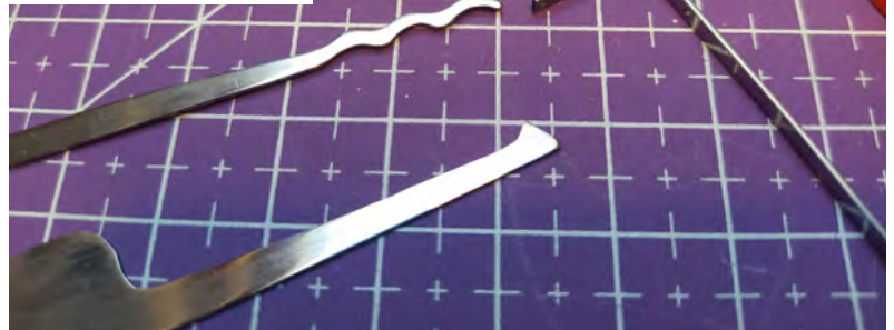
Above ♦ Our small collection of completed tools: two tension wrenches, a half-diamond pick, and a double-ended 'Bogota'-inspired rake
