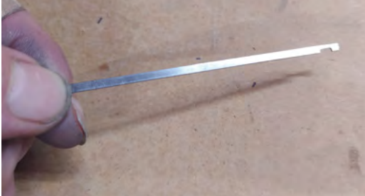
Figure 2 ♦ This small stainless steel strip has been removed from a discarded windscreen wiper blade
