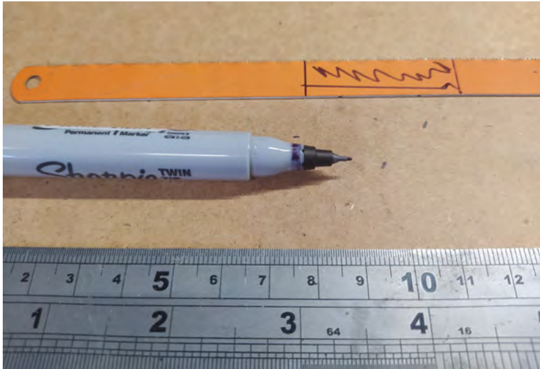
Figure 5 ♦ Again we used a thin permanent marker and a ruler to mark our design onto our hacksaw blade blank
