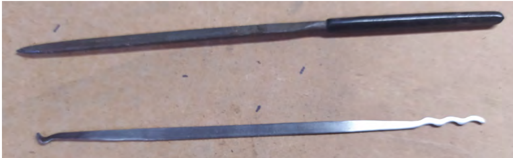
Left ◆ Bogota rakes made from sweeper bristles are relatively easy to make using a small file instead of grinding tools if they aren't available
