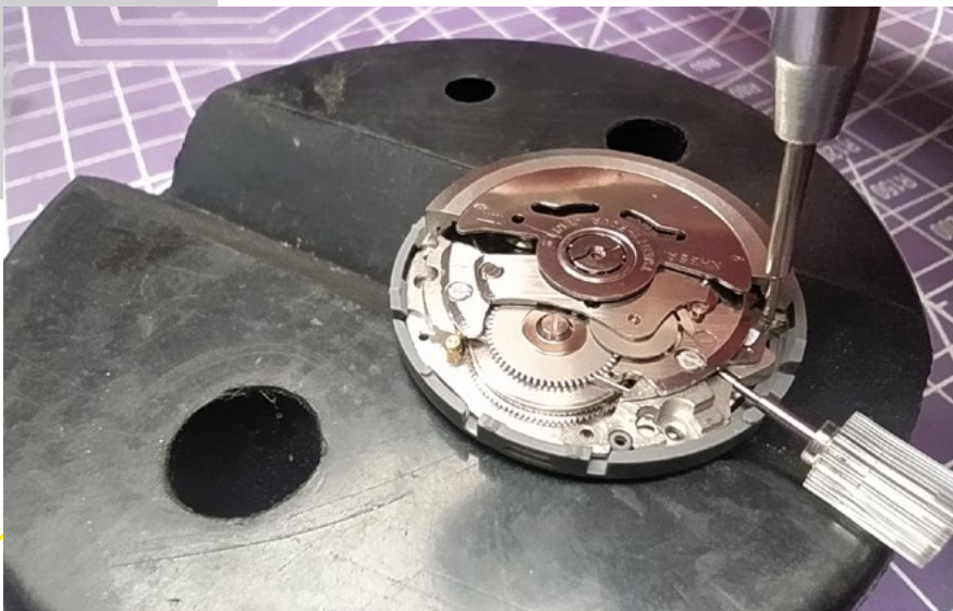
Below ⬇️ Using a small pin tool to release the dummy stem from the movement
