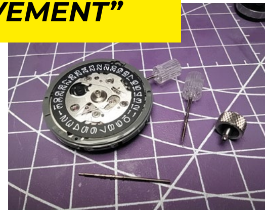
Figure 1 ↗ An NH35 movement with a dummy stem and crown; an oversize stem was also supplied with the movement
