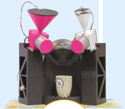
◆ The K-Fee comprises numerous 3D-printed parts, including funnels to hold the coffee and sugar
