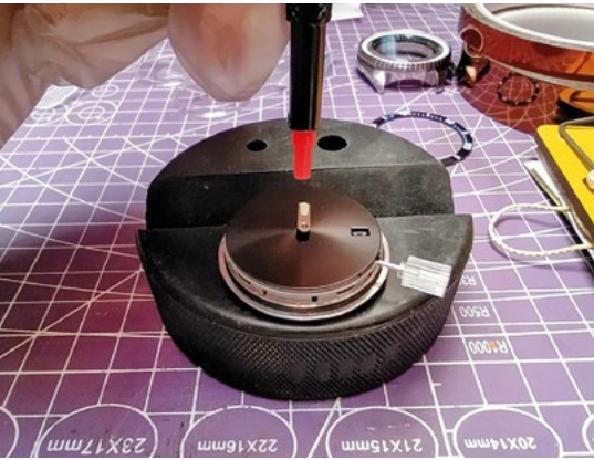
Above ⬆️ Using the correct hand fitting tool and tweezers, you need to exercise extreme care in handling and fitting the hands
