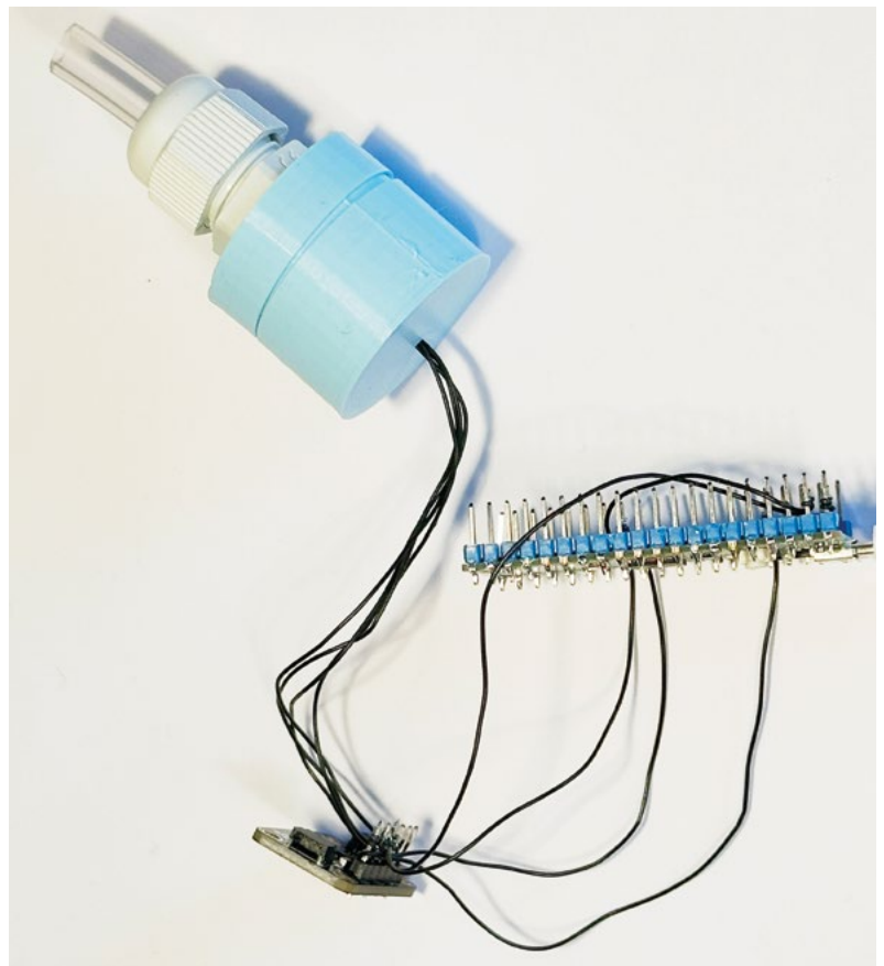
Figure 5 ♦ The pressure sensor is connected after the distance sensor on the same I2C connection
