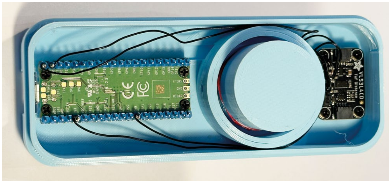
Figure 8 ♦ The pressure sensor fits inside the pipe
