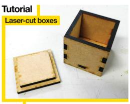
Zap plywood to turn it into bespoke project enclosures
