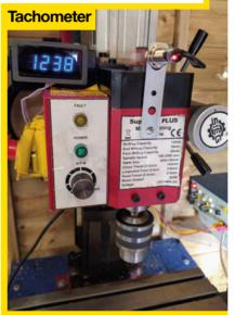
An inexpensive Hall effect sensor to keep track of rpms
