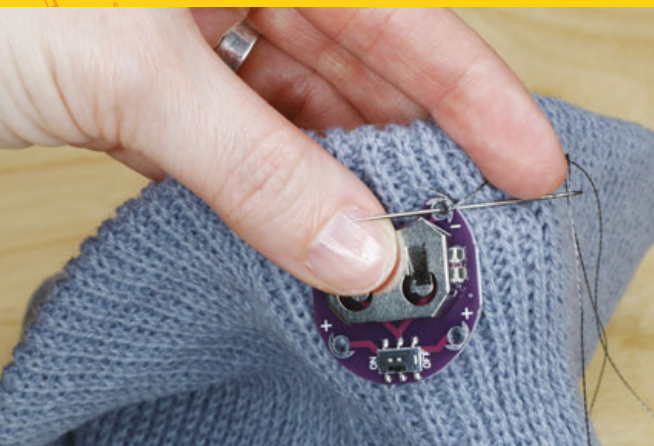
Below ♦ The battery holder should go along the side of the hat, where it will fit along the side of your head
