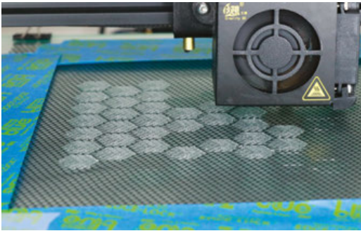
Above ♦ 3D-printing the panels on fabric
