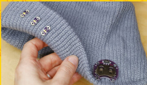
Above ♦ The battery holder lives on the inside of the folded-up part of the hat, its unsightliness hidden
