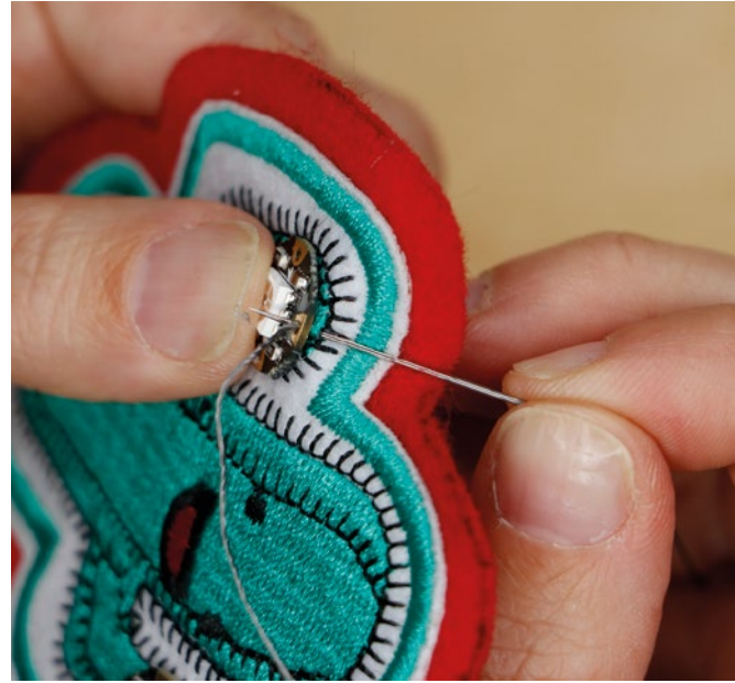
Above ♦ Connect the NeoPixel with conductive thread
