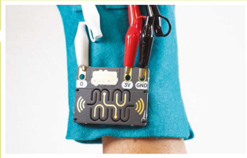
Left ♦ Short crocodile leads are easy to connect and stay in place during use
