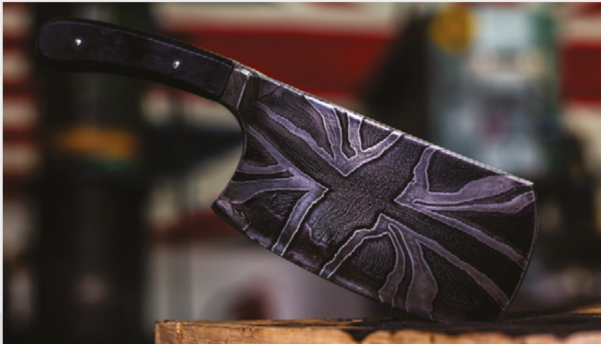
Left ♦ This Union Flag is in the steel itself, an effect achieved through careful beating and cutting
