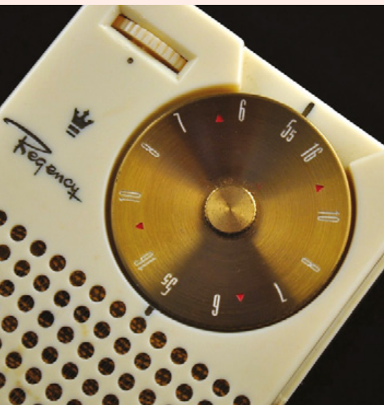
Left ♦ The Regency TR-1 from 1954, the world's first commercial transistor radio
