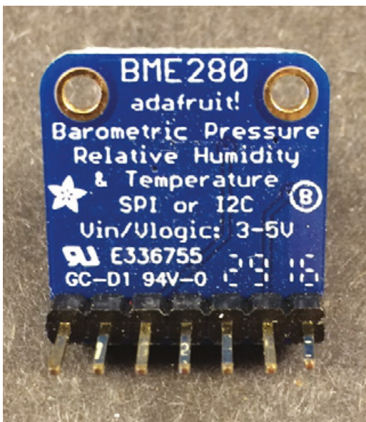
Figure 1 Although not as reliable, you can leave the header off and press-fit wires into the holes to avoid soldering
