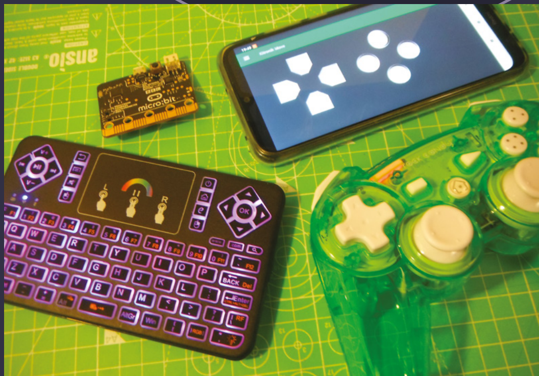
Left Numerous controllers for robot projects including a micro:bit, a Rock Candy PS3 gamepad, the Kitronik Move app, and a small wireless keypad
