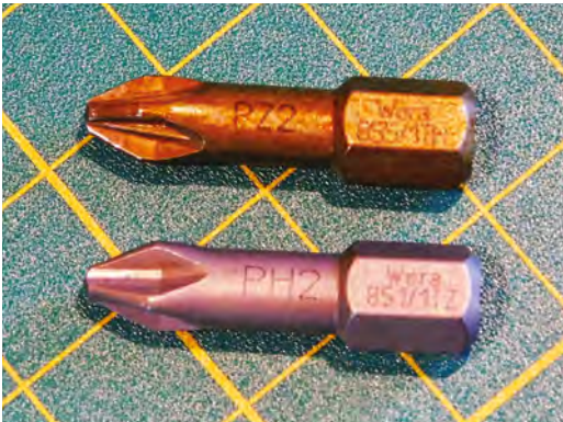
Above ♦ Pozidriv (top) and Phillips (bottom) look similar, but you'll have problems if you use the wrong driver for a screw
