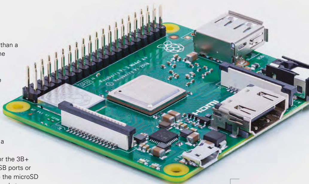
Above □ The camera and display connectors can be used with the official hardware to add a visual aspect to your makes
