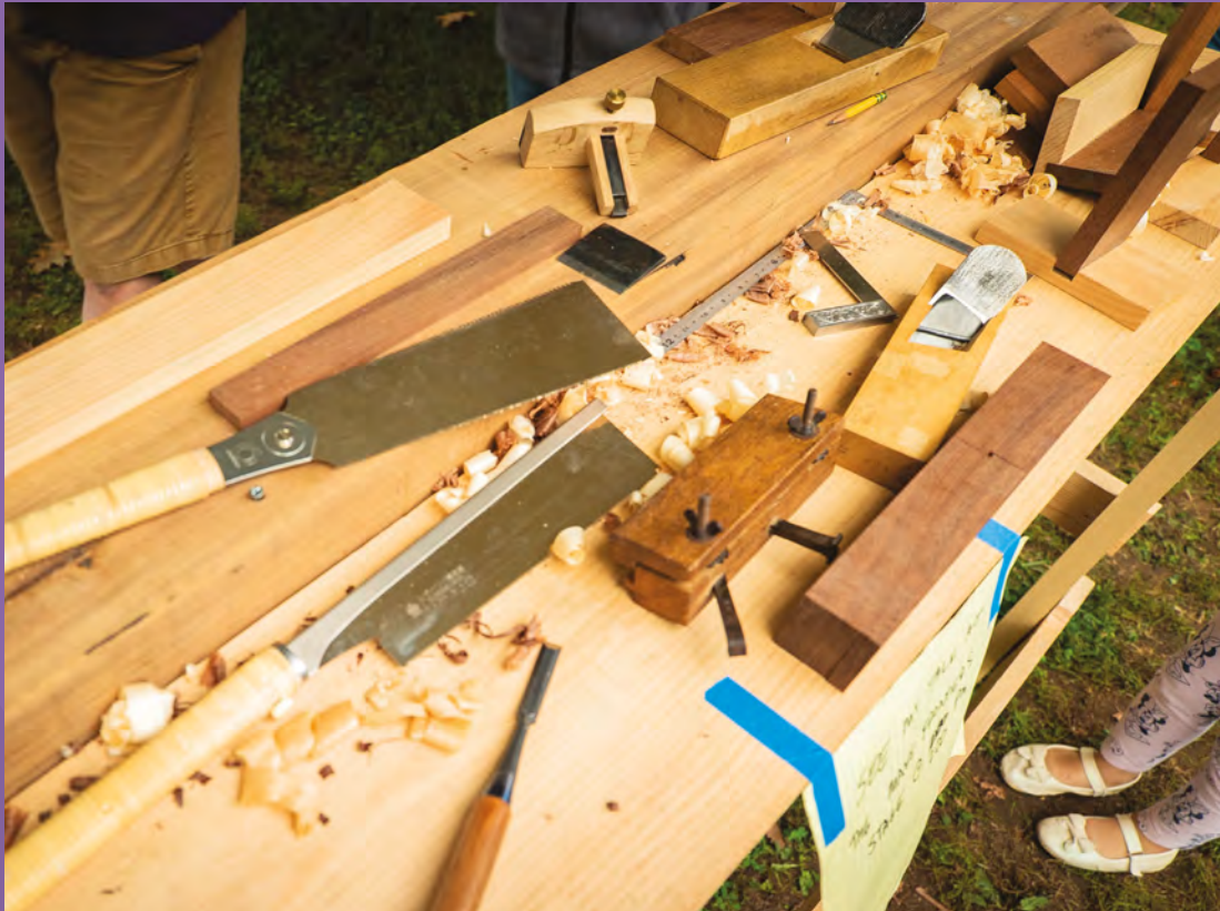
Left ↔ Like the saws, Japanese planes work with the pull stroke, and remove less wood than a typical Western plane
