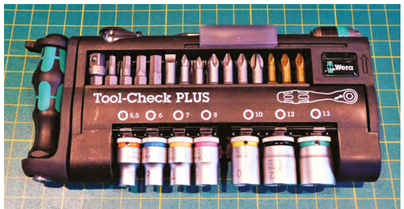
Below □ The Wera Tool-Check Plus will work with all common screw types and folds down into an easy-to-transport pack
