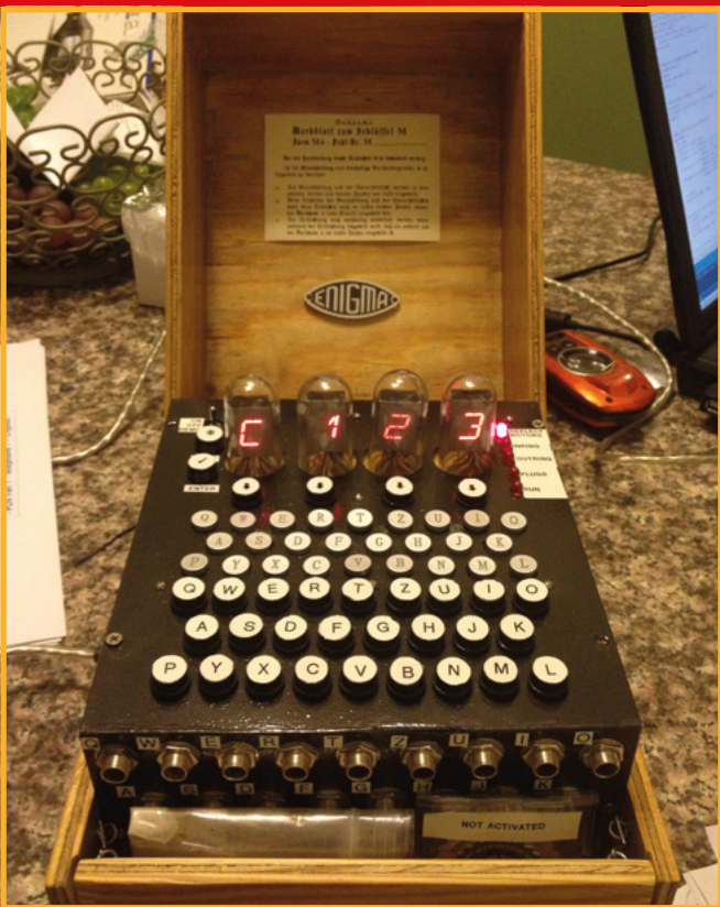
◆ While this looks like a hardware project, much like the real Enigma, the brain of this replica is actually software
