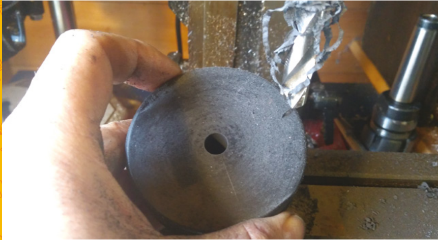
Figure 4 ♦ Drilling the hockey puck central 10 mm hole was the first time we had cut rubber. Note the large amount of dust it produces!
