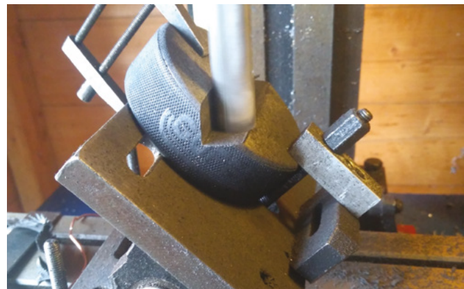
Figure 6 ♦ Cutting the groove with an end mill with the hockey puck creatively clamped to the angle plate
