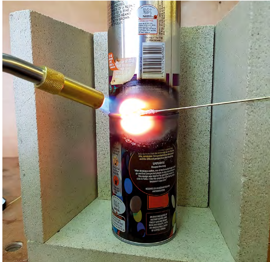
Above ♦ Get the joining surfaces hot, and use them to melt the brazing rod. Try to keep the heat even, so that the surfaces don't warp too much
