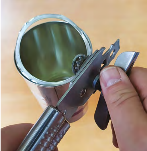
Above and right ♦ ♦ Clean paint from the cans with a wire brush to get the best joint, and remember to cut the bottom out of the can before you braze it in place
