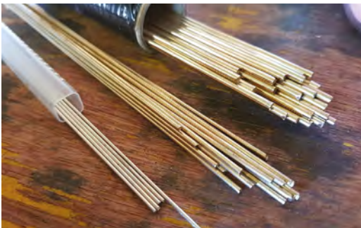
Above ♦ It's best to keep your brazing rods labelled, as different alloys can look very similar to each other. Here, you can see silicone-bronze (top), brass (middle), and 55% silver rods (bottom)
