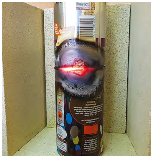
Above ♦ Get the joining surfaces hot, and use them to melt the brazing rod. Try to keep the heat even, so that the surfaces don't warp too much
