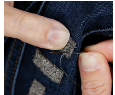
Above Left ■ To hide the circuit, sew the conductive thread along the jacket's stitch lines
