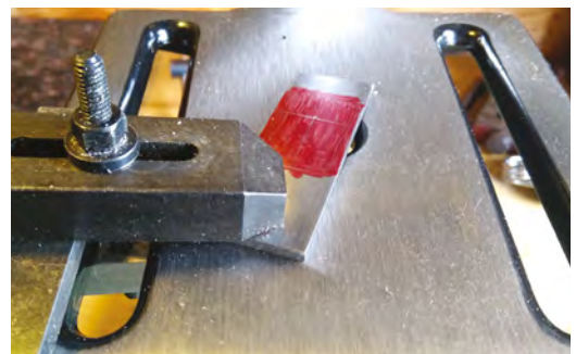
Figure 2 ♦ Using milling clamping accessories to clamp a workpiece
