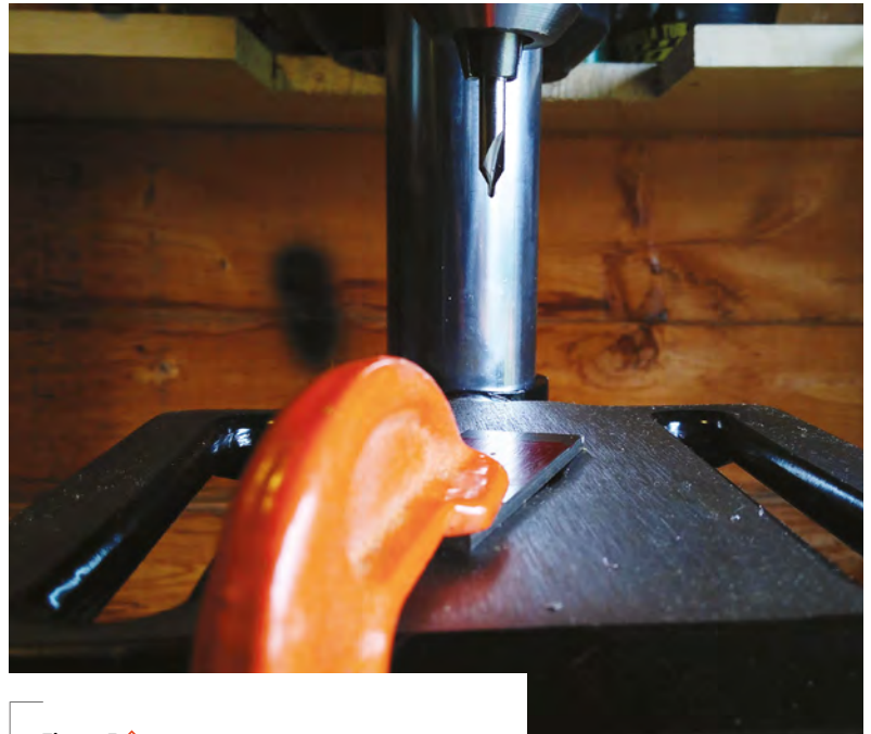
Figure 3 ♦ Using a G-clamp is a good budget way to clamp work securely. The centre drill is already mounted in the chuck to begin to drill accurately
