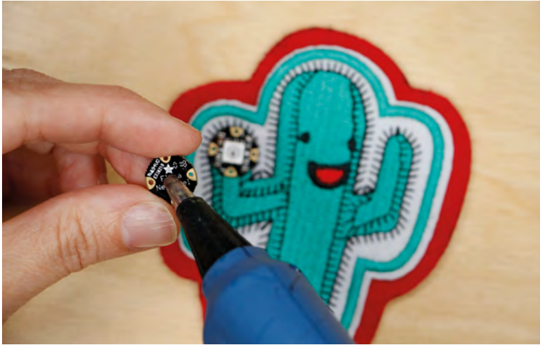
Above ♦ Hot-glue each NeoPixel into place on the patch
