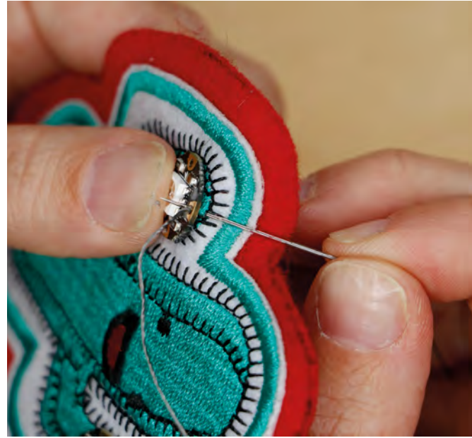
Above ♦ Connect the NeoPixel with conductive thread
