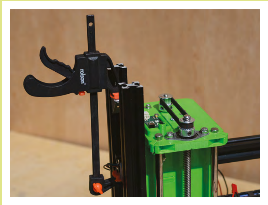
Above ♦ Holding the mill together while it's assembled
