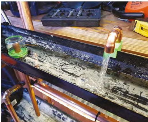
Above ♦ The system under test, showing water flow from the outlet, and the greedy cup mechanism on the left of the photo
